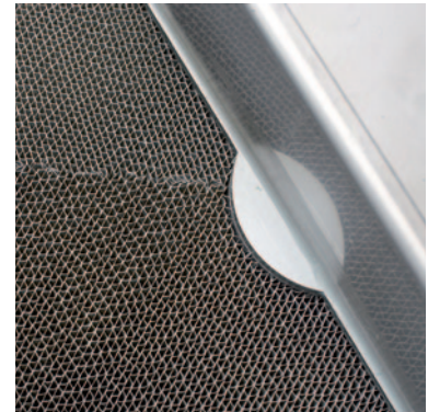
The rotor adsorbs moisture on the silica gel covered surface while it is in the drying zone. In the regeneration zone the moisture is released and the rotor is ready for another turn in the drying zone.
